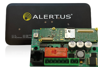
Alertus Text-to-Speech Interface provides clear spoken voice output of message text
